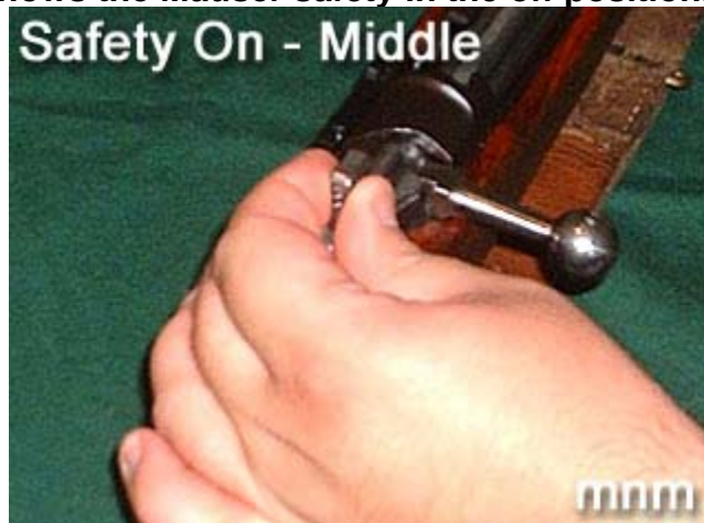
Safety 2 shows the Mauser in the middle position. This position allows for the opening of the bolt - but does not allow for the trigger to be pulled.
