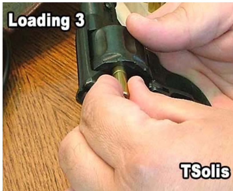
Figure Loading 3 shows inserting a single cartridge. Then the cylinder is rotated and each empty chamber is loaded. Once finished the loading gate is closed and the pistol is ready to be fired.
