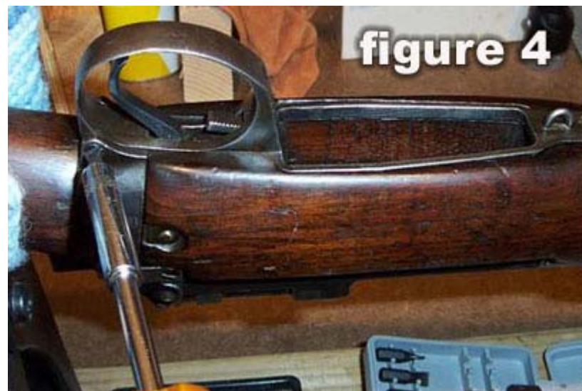
Figure 4. Removing the rear screw of the trigger guard.
