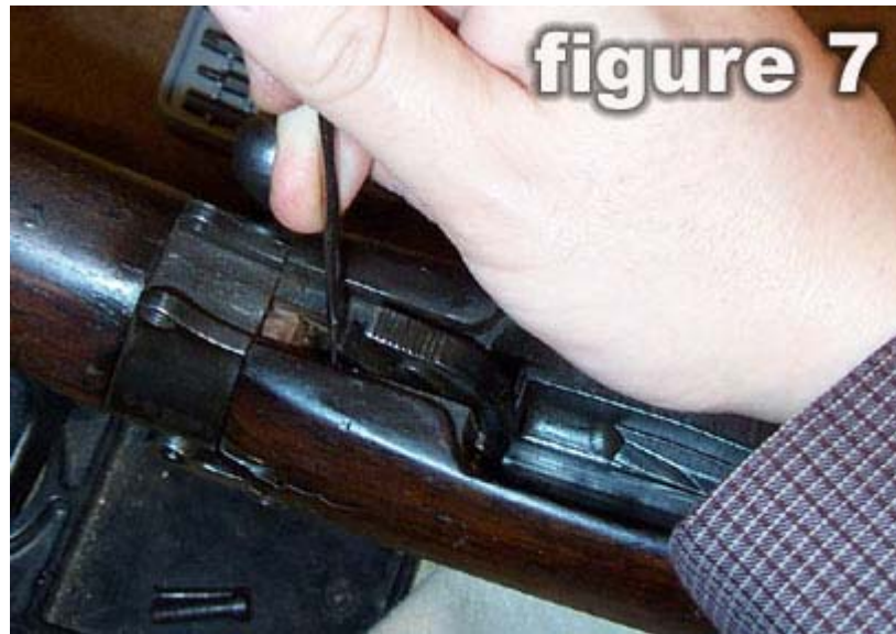
Figure7. A small screwdriver helped immensely when re installing the trigger/trigger guard. Push sear forward and then slip ball bearing under sear, seating rear of trigger guard first, then the front. Photo is without guard in place.
