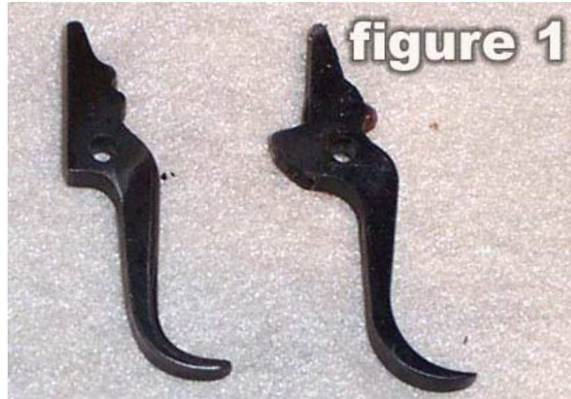
Figure 1. Left is the original Enfield trigger out of my No4. Mk1. Left is the Huber trigger. Note the ball bearing and shape difference.
