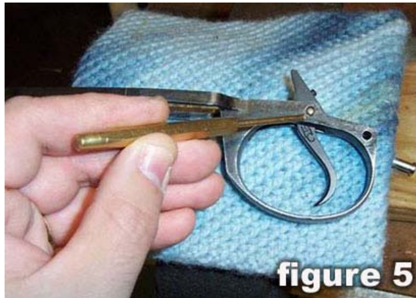
Figure 5. One pin to drift out. You do not even have to drift it out completely. Use a brass punch to protect the metal.
