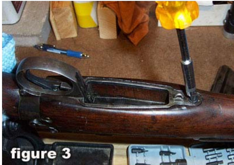
Figure 3. Removal of the front screw holding the trigger guard in. Make sure that you do not lose the split spring ring under the screw.
