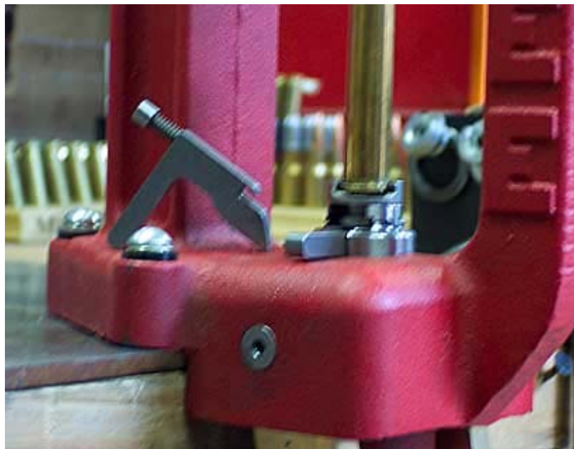
Primer Being Seated In a 30/06 Case
