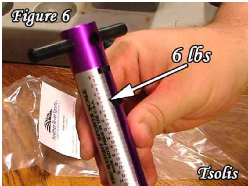
The 98k's trigger only measured 6lbs!
