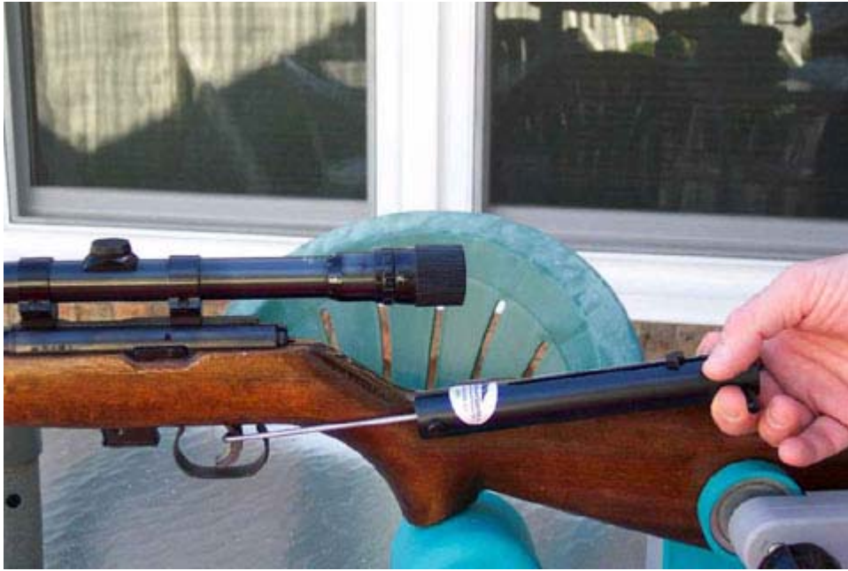
Measuring trigger weight with Feather River Sports 10 lb gauge on the 1969 Romanian .22 rimfire trainer.
