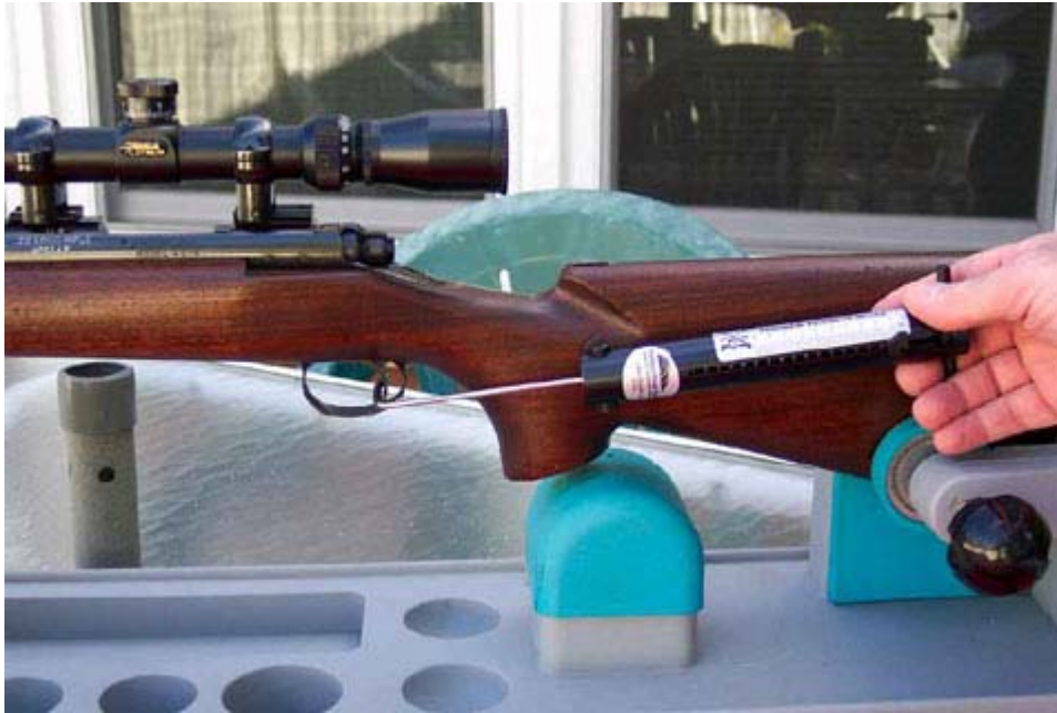
Measuring trigger weight with Feather River Sports 8oz - 10 lb gauge on the Remington 40X .22 rimfire match rifle.
