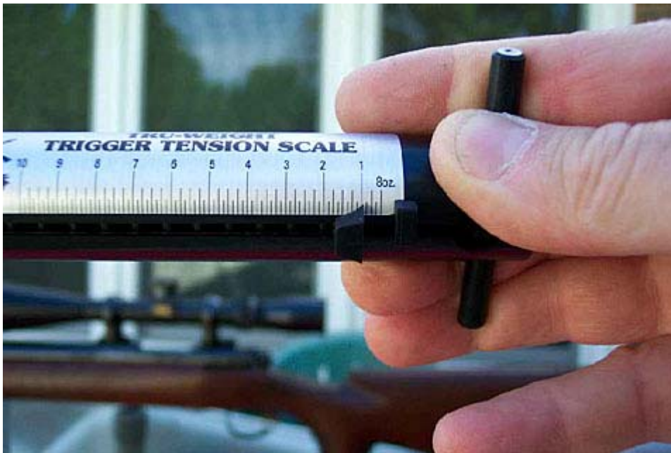
Feather River Sports measured a 1 lb pull on the slick triggered Remington 40X.
