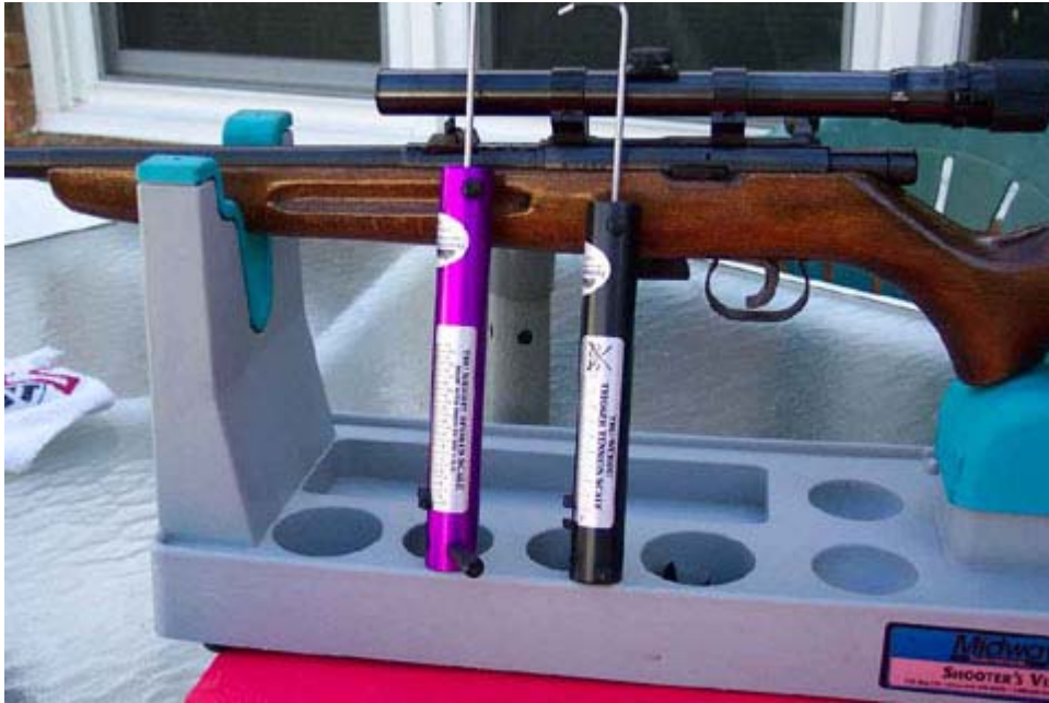
Feather River Sports Trigger Pull Gauges: 0-25 lb gauge on left, 8oz. To 10lb gauge on right
