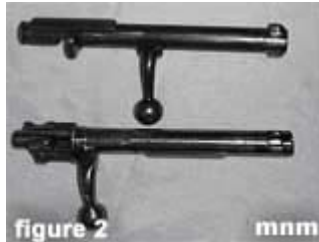
Figure 2: side by side comparison of a Mauser 48A (bottom) and Carcano bolt.
