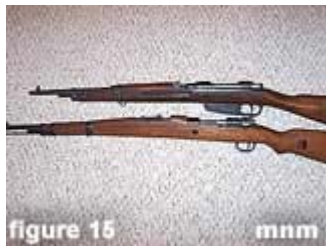
Figure 15: A side by side comparison of length between the M38 Carcano and M48A Mauser. The Carcano barrel is shorter by about 3" and the rifle is considerably lighter. Both factors lead to a more pronounced muzzle blast and felt recoil.
