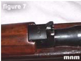
Figure 7: Fixed rear sight is set for 200m. Note stamped caliber "6.5mm" on sight.
