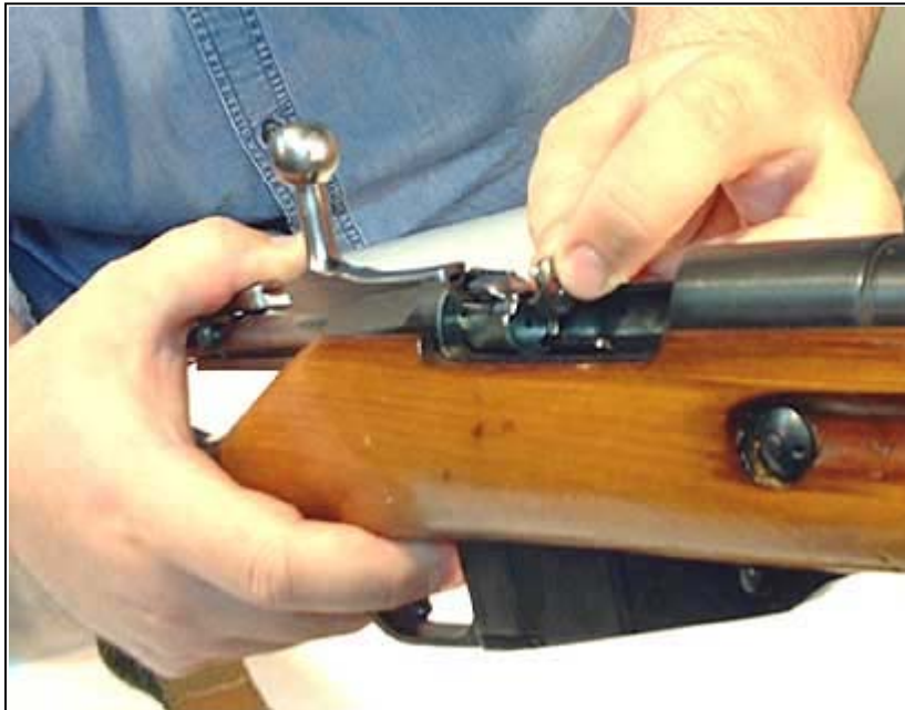
Inserting a Yankee Engineers "No-Go" gauge into a 7.62x54r Mosin-Nagant.
