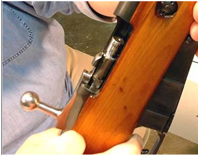
Inserting a Dave Manson Precision "Go" gauge into a 7.62x54r Mosin-Nagant.
