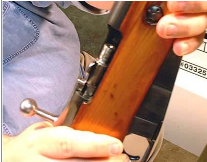
Inserting a Dave Manson Precision "No-Go" gauge into a 7.62x54r Mosin-Nagant.
