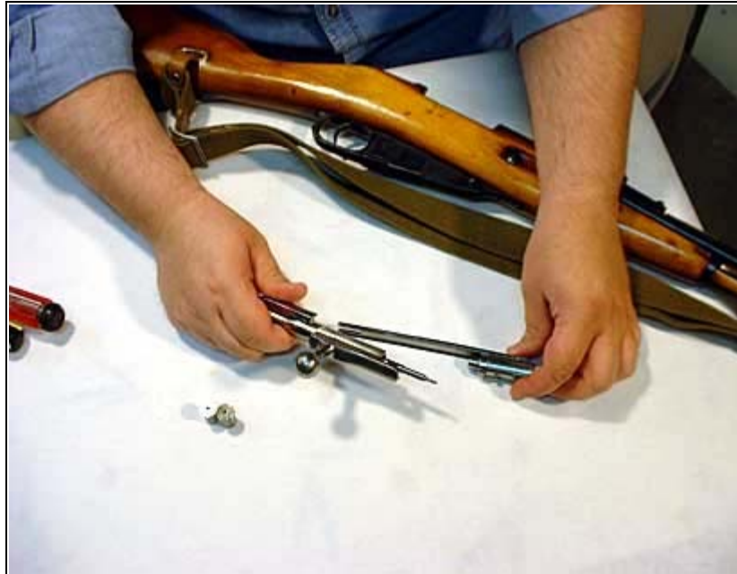
Separating the Mosin-Nagant bolt assembly to remove the firing pin and firing pin spring.
