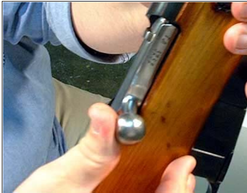
The bolt successfully closes on the "Go" gauge.
