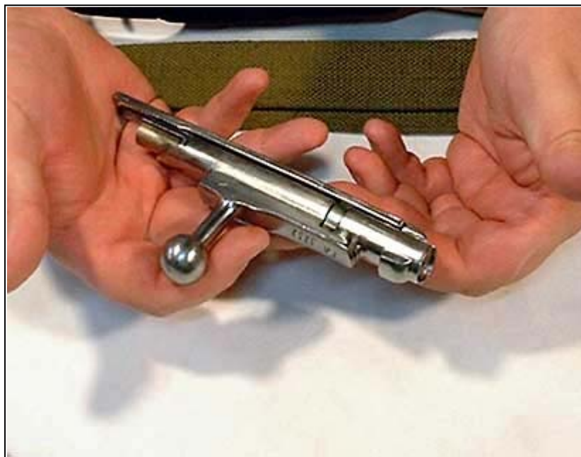
The reassembled bolt minus the cocking piece, firing pin, firing pin spring, and extractor.
