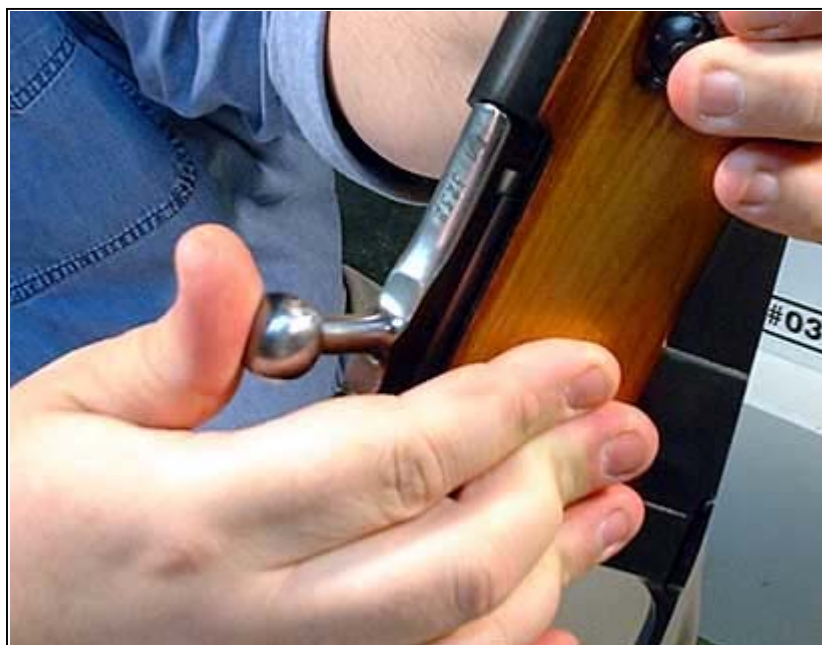
The bolt does not close on the "No-Go" gauge. Note: Do not force the bolt closed.
