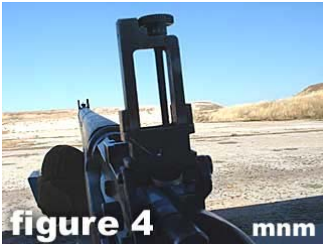
1st Variation Backsight Leaf Sight with 300 yard battle sight and leaf graduations of 200 to 1300 yards.
