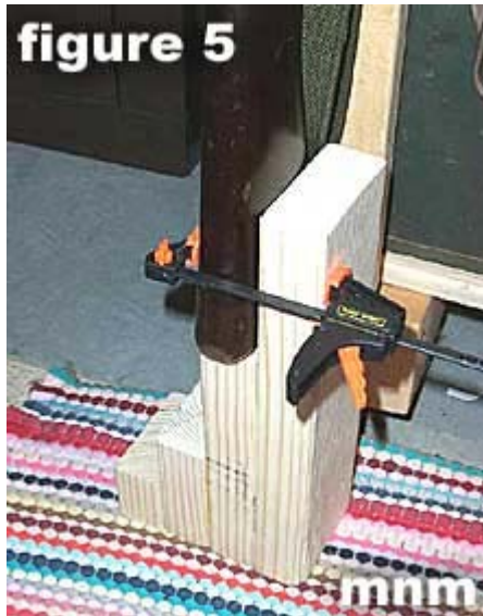
Figure 5. A couple of different lengths of 2x4 and a clamp provide a nice step block to support the stock when working vertically.
