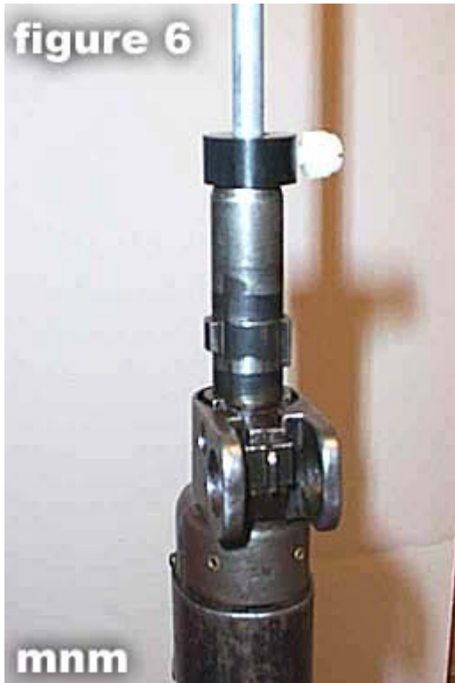
Figure 6. Make sure that the cleaning rod stop is flush against the muzzle of the rifle before tightening it down.
