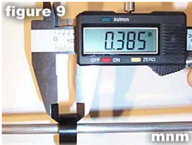
Figure 9. Note that the thickness of the stop was measured at the same point where the total length was measured from.
