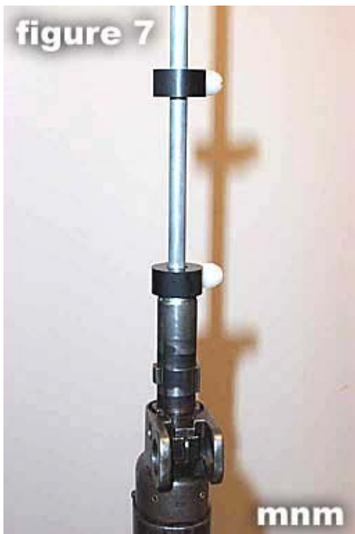
Figure 7. As with the first cleaning rod stop, make sure that the stop is flush against the muzzle of the rifle.
