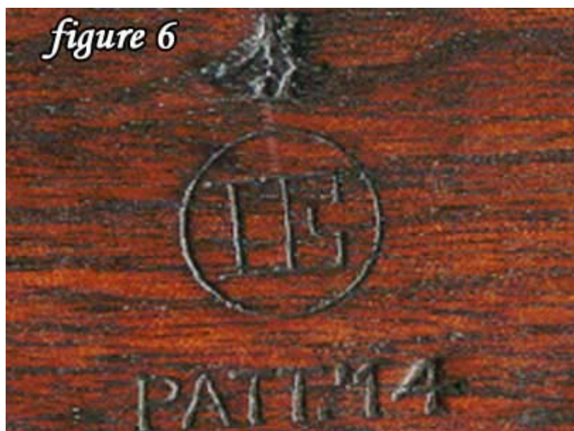
Eddystone Mk I Pattern 14 Rifles were Stamped with IE on the Stock inside of a Circle. The I representing Mk I and the E representing Eddystone.
