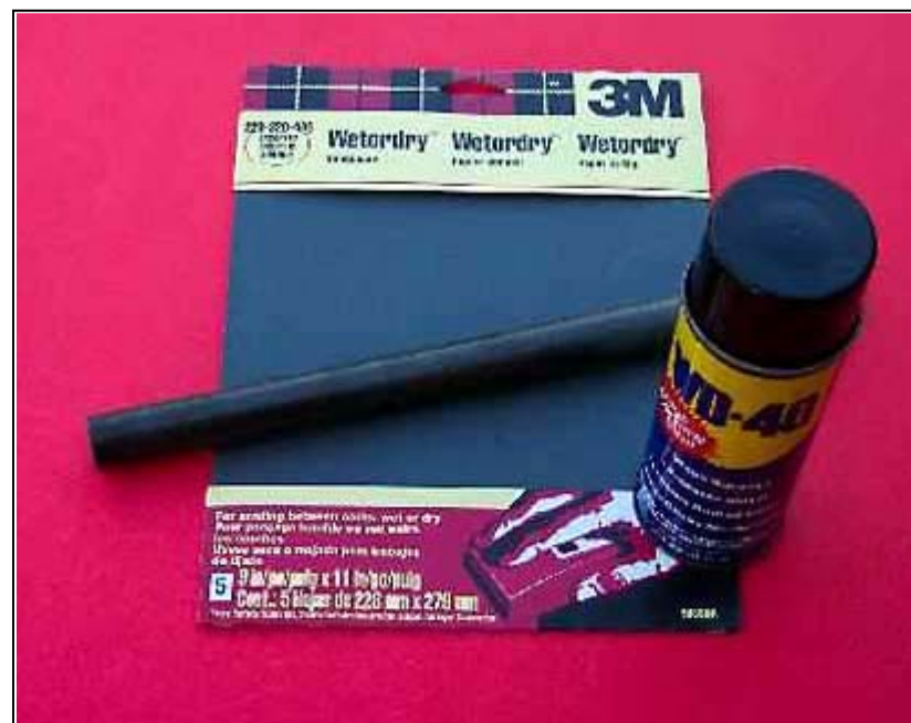
Lapping Materials For Cheap Guys: Wetordry Paper, 1 inch Thick Metal Bar, WD40; Total Cost; About $8.00
