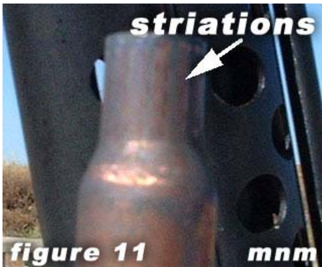
Striations or flutes left on spent case from fluted chamber
