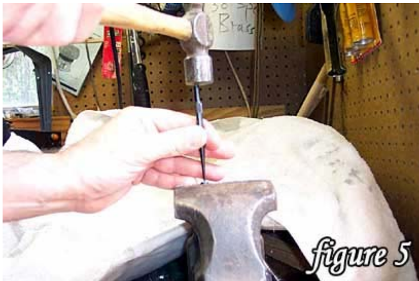
Center punching sight base, make sure you hit in the exact center of where old, tapered post was
