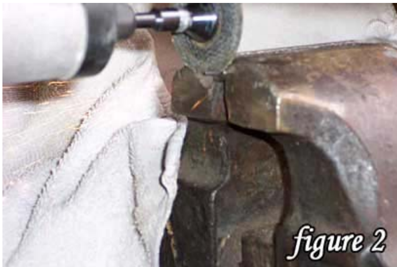
Impregnated cut-off wheel on Dremel tool removes tapered post from sight base.
