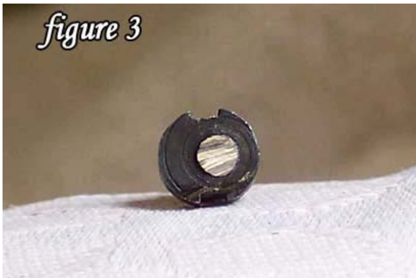
Sight base after tapered post has been cupped off
