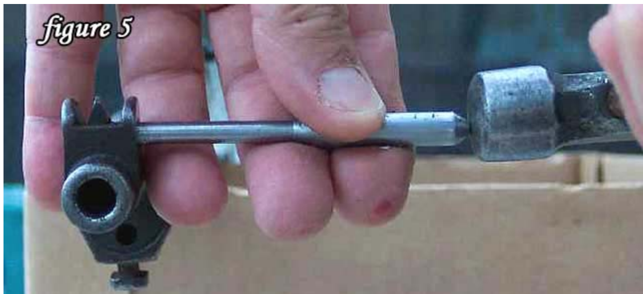
A hammer & drift pin is OK, but be careful!
