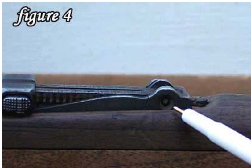
Make sure the pin & holes aren't worn where the sight pivots.
