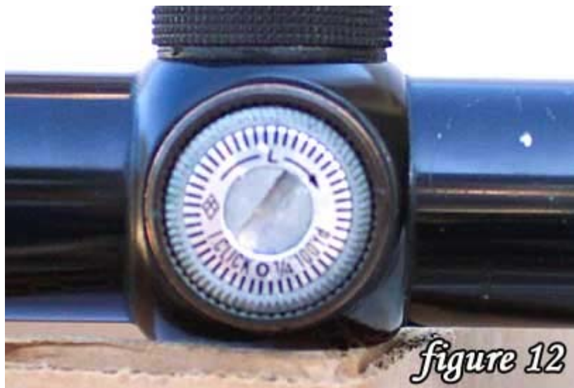
The adjustment turret of a Tasco (Japan) 4X sporting scope.
