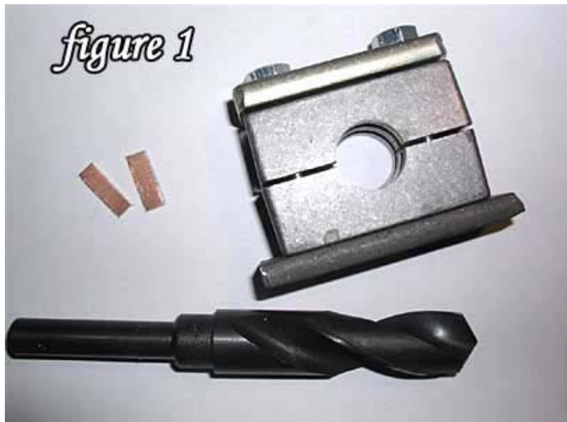
Parts needed for launcher removal: clamp, 55/64" drill bit and two scrap pieces of printed circuit board.
