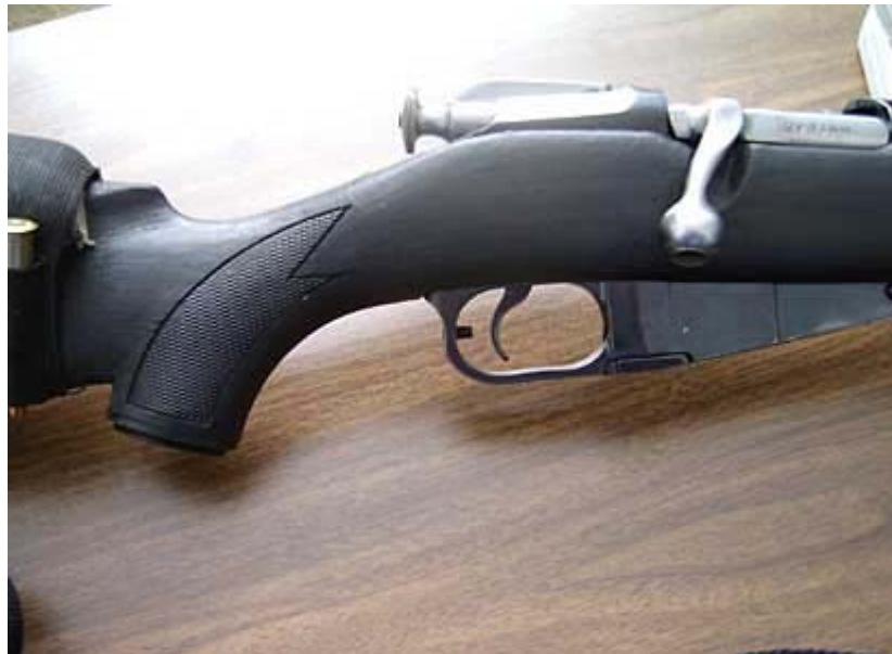
A picture of the trigger over travel stop. It's really just a blued piece of 10/32 screw, but it sounds cooler to call it a "Over travel stop"
