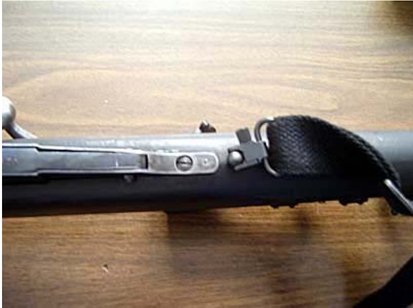
The placement of the third sling swivel just forward of the action. The short sling is attached here.
