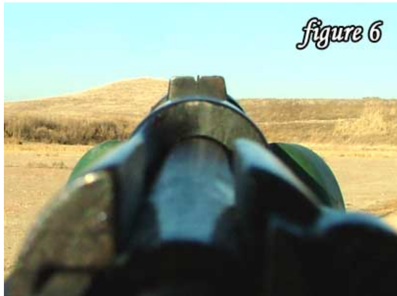
The front sights were modified to have higher blades to provide for a zeroing distance of only 150 meters.
