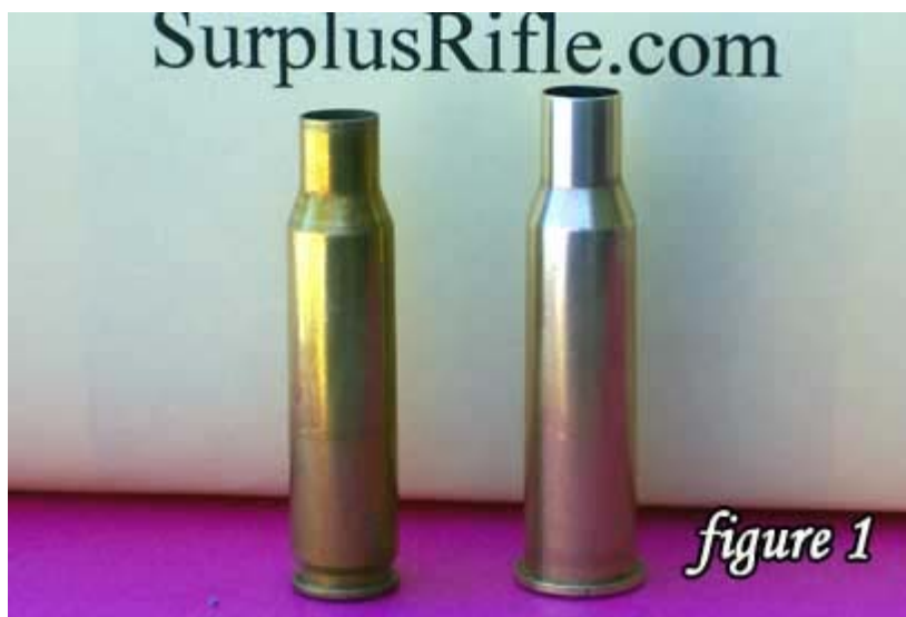
The 7.62X54R is .099 longer than the .308 Winchester
