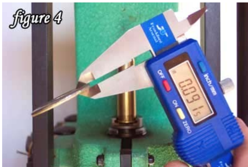
The washer is .091 thick. This will take up most of the case size difference
