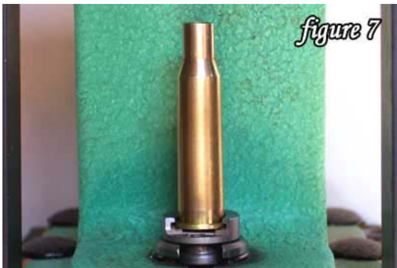
7.62X54R inserted in the shellholder
