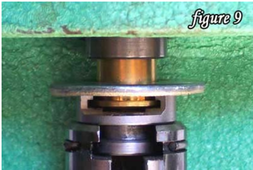
Washer is approaching the sliding sleeve of the LEE .308 Collet Die
