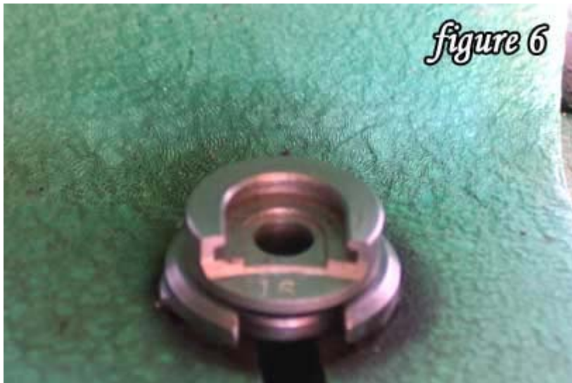
LEE shellholder # 16 is correct for the 7.62X54R
