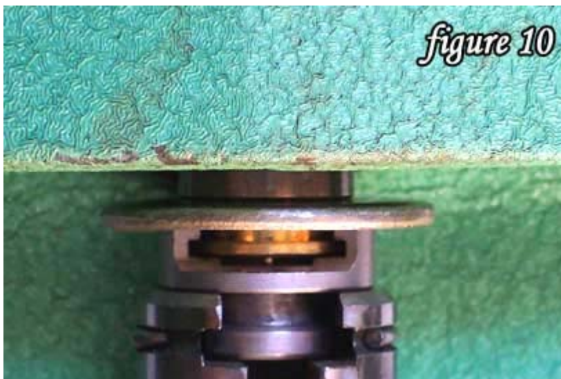
Washer is pushing up on sleeve, collet is closing
