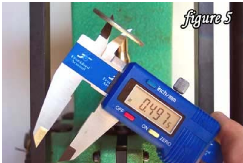
The hole in the washer about ½ inch, common hardware store fare
