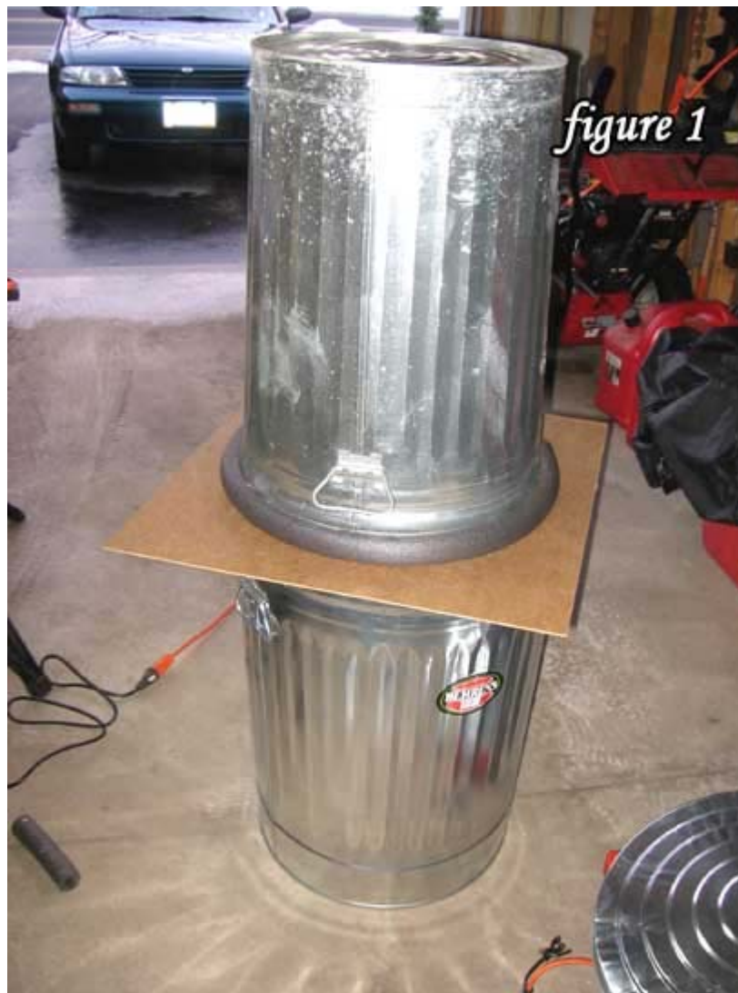
The entire contraption. The 20 gallon is supported by the particle board cut to a smaller diameter.
