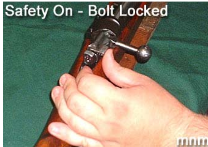
Safety 3 shows the Mauser in the far right - "Safety On" position. This position does not allow you to open the bolt or pull the trigger. Sights
